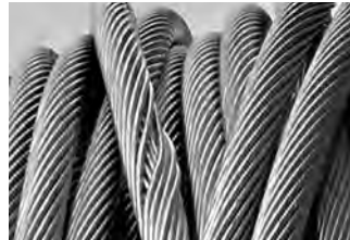
Figure 7 – T-2 ® Damage due to Excessive Brake Tension on Pay-off Reel
