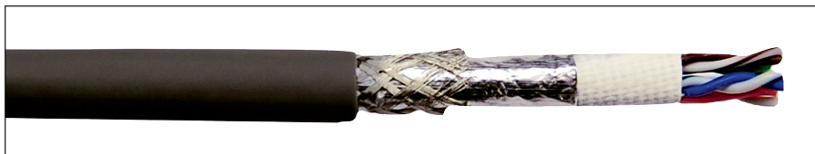
TRANSIT, 4 PAIR/24 AWG, SHIELDED FOIL TWISTED PAIR (SF/UTP) CAT 5e, LOW-SMOKE, ZERO-HALOGEN
