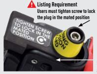
Zone 2/Division 2 DR50 receptacles feature a standard screw-type locking pawl. This required feature allows the user to lock the plug to the receptacle by tightening a screw on the pawl.
